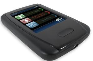
The DataPad allows users of FilesThruTheAir™ USB data loggers to configure their units and download data and view logging results on-the-spot rather than removing the logger from the environment being measured and taking it to their PC. This allows continual logging with shorter breaks in data collection, less travel for the user, on-site data collection in graph, legend and summary format and the ability for users to reconfigure loggers in 'the field'.
